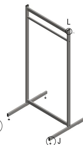
**3** COM A ARARA EM PÉ, APERTAR OS PARAFUSOS ATÉ O FINAL. NIVELAR E AJUSTAR ALTURA ATRAVÉS DOS PÉS NIVELADORES.
