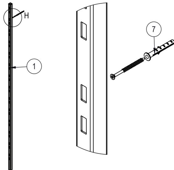
**2** FURAR NO LOCAL DA MARCAÇÃO (FURO DE 6MM) E INSERIR BUCHA CONFORME TIPO DE PAREDE (7 OU 8). UTILIZAR O PARAFUSO (6) PARA FIXAR A COLUNA NA PAREDE.
